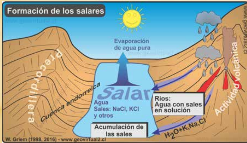
Figure 3: Formation of a salt flat. The high evaporation rate allows the accumulation of large masses of salt (taken from www.geovirtual2.cl ). In particular, the high concentration of chemical elements such as sodium (Na), potassium (K), chlorine (Cl), lithium (Li), and boron (B), among others, in the waters of high Andean fluvial systems triggers precipitation and crystallization into minerals such as halite, sylvinite, and bishovite. Lithium salts and borates are also found. A good example is the Salar de Pedernales; Figure 4 shows the real dimensions of this area.
