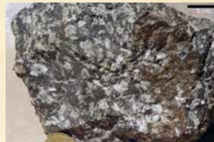
B) Andesite: Volcanic rock with porphyric texture. Very common in the Mesozoic at the foothills
